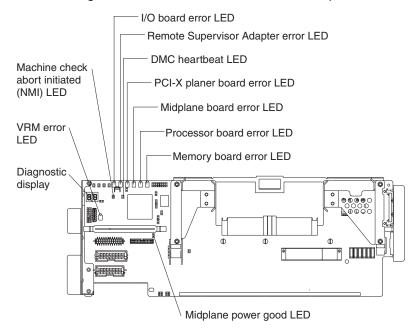
You can see the midplane board LEDs on the top of the server. These LEDs are numbered from 1-6 and indicate the board on which an error has been detected.
